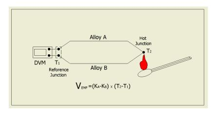
Because it is very difficult to predict the thermal EMF coefficient of an alloy from its element composition, all the values for materials commonly used are obtained by measurement. Measurements are made by fixing the material of one of the elements to a common metal such as platinum or copper. Thus the thermal EMF coefficient for each metal is stated as referenced to the same reference metal.
