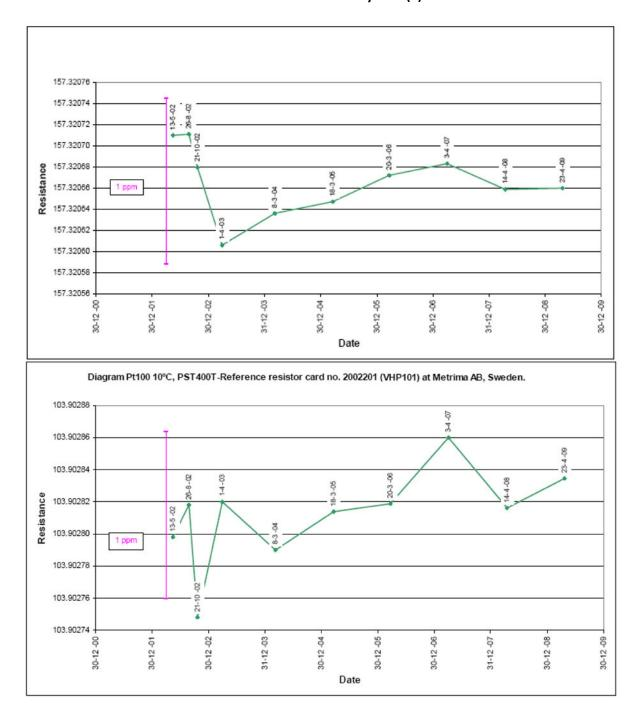
(\*):ΔR/R Data is available for 30 years shelf-life in non hermetic resistor at non controlled atmospheric conditions is in the range of 25 ppm
