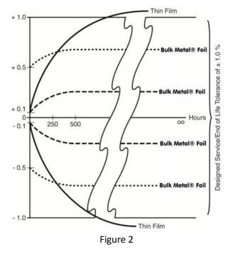
At the zero-hour point shown on the graph, the resistor has been placed in service in the end equipment. Up to this point, a number of degrading factors (such as those shown in Figure 1) will already have occurred and exacted a toll on the purchased tolerance. These contribute to the rapidly rising curve, but probably would not be "seen" until turn-on time.
