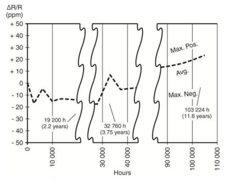
Figure 3: S102C (Bulk Metal® Foil Resistor)  $1k\Omega$  over 10 years, actual tests.
